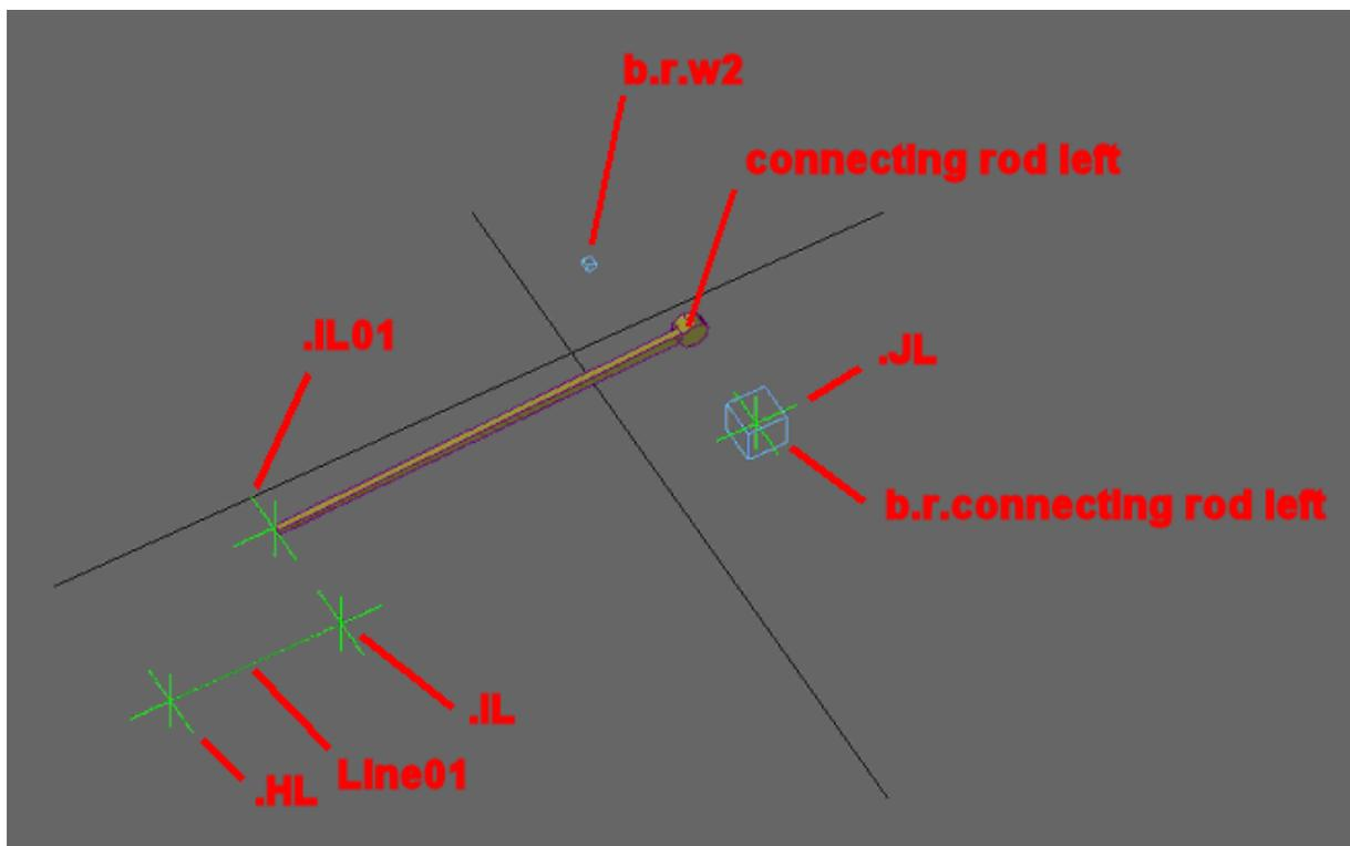
It's not as bad as it sounds actually. Create dummy called ,b.r.connecting rod left' in top view and align it in X,Y and Z to point ,.JL'. Create a line ,Line01' between ,.HL' and ,.IL'
