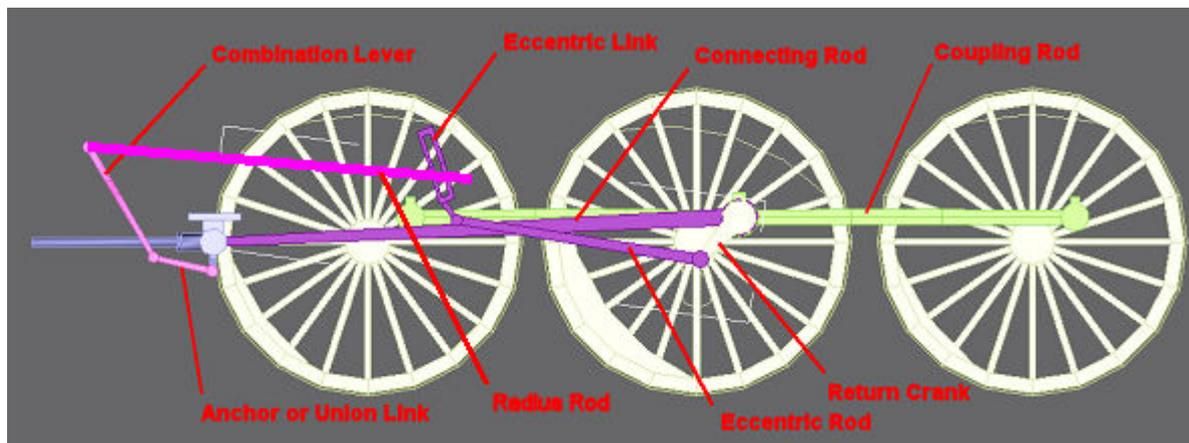
By the way, when the loco is in forward gear the joint between the Radius Rod and the Eccentric Link is below the pivot point of the Eccentric Link, and when in reverse gear above it. In real models (and most virtual ones!) a common dodge is to model the gear in 'neutral', i.e. the Radius Rod pivot is coincident with the Eccentric Link pivot. This means that the Radius Rod doesn't move which is a pity.
