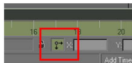
Under ,Customise -> Preferences' change the ,Precision' to 4, ,Snap' to 0,01' and select ,Use Snap'. This enables finer control over the spinners for moving/rotating objects.
