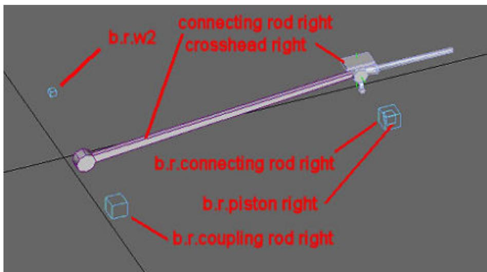
The first step is to link 'b.r.coupling rod right' to 'b.r.w2'. Hide everything you are not working on and use the 'Link' tool to create links between the objects by dragging.
