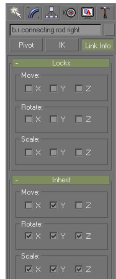
Link 'b.r.piston right' to b.r.connecting rod right'. In the 'Hierarchy' tab set the 'Inherit' and 'Move' check boxes for 'b.r.piston right' as shown.
