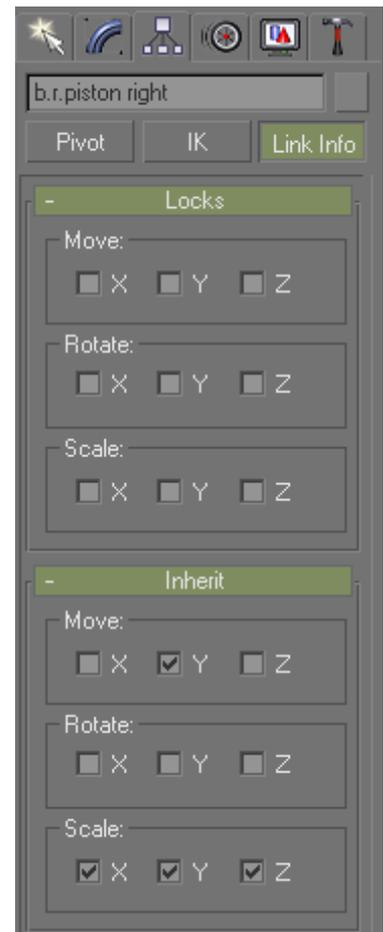
Link 'crosshead right' to 'b.r.piston right' and 'connecting rod right' to 'b.r.connecting rod right'. The tree should look like this now: If you play the animation now you'll see that the connecting rod is animated but doesn't point to the crank pin on the driving wheel, this is where the 'LookAt' constraint comes into play.
