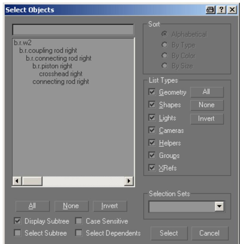
Select 'b.r.connecting rod right' and in the 'Motion' tab choose Parameters -> Assign Controller -> Rotation'. Click on the 'Assign Controller' icon (the green arrow under the text 'Assign Controller').
